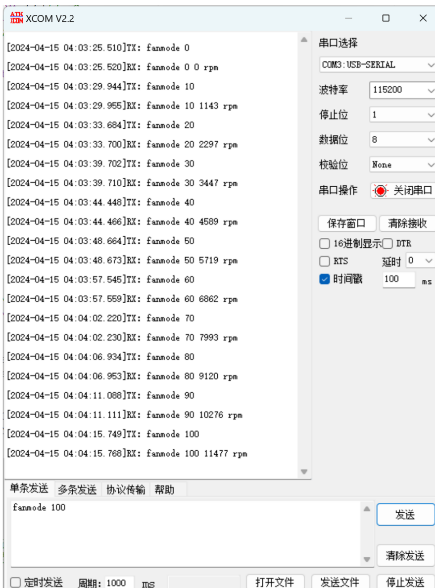
图 6-9 散热器控制测试 Figure 6-9 Radiator Control Test
